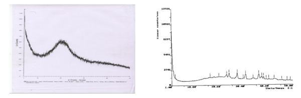
Figure2.a. and 2.b: X-ray diffraction study of tamarind fruit and seed
